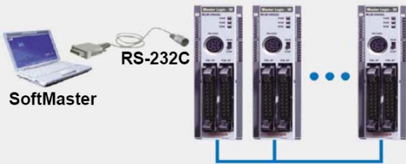
Remote connection using RS-485 Communication
