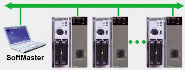
Remote connection using Ethernet
